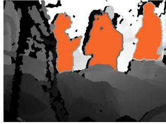
**Fig. 2.** Personnel are segmented from the depth images and placed into individual action sequences.
