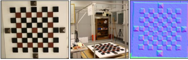
Fig. 2. A 3D checkerboard target used for ideal characterization (left), example experimental setup (LMS291 shown) for scanning the checkerboard (middle), and a mesh model of checkerboard generated using range data (right).
