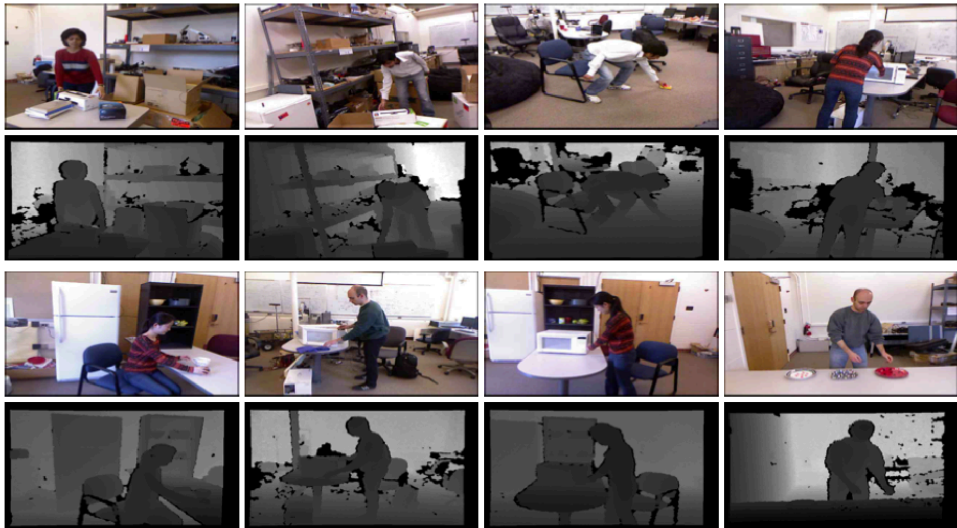
Fig. 2. Significant Variations, Clutter and Occlusions: Example shots of reaching sub-activity from our dataset. First and third rows show the RGB images, and the second and bottom rows show the corresponding depth images from the RGB-D camera. Note that there are significant variations in the way the subjects perform the sub-activity. In addition, there is significant background clutter and subjects are partially occluded (e.g., column 1) or not facing the camera (e.g., row 1 column 4) in many instances.
